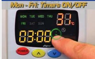
**2** Adjust the hours you require by using the **▲** and **▼** buttons. Immediately press the green set button again to get to the minutes and use the **▲** and **▼** buttons to adjust the minutes.
