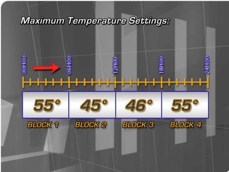
**1** To adjust the maximum temperature settings, press the green set button until the first block temperature setting is displayed. The temperature will be flashing and the number of the block will be displayed in the timer indicator block. The below screens show the temperature flashing in block number 1.
