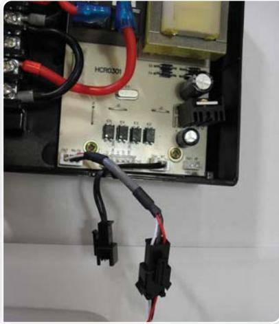
**STEP 4: Remove thermostat and replace with supplied geyser temperature probe**
