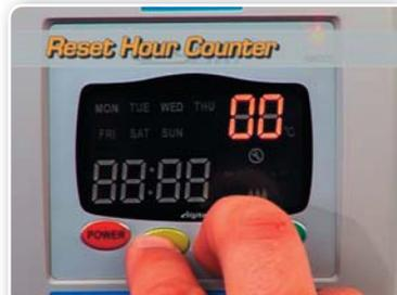
To reset the hour counter, keep the up and down arrow buttons in simultaneously until the main time settings reappear.
