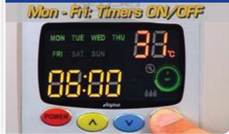
**4** Adjust the hours you require by using the **▲** and **▼** buttons. Immediately press the green set button again to get to the minutes and use the **▲** and **▼** buttons to adjust the minutes.
