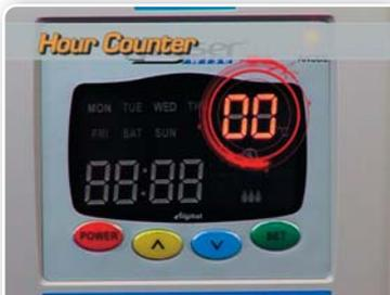
For example: Let's say the hour indicator indicates 30 hours. You then multiply the number of hours with your geyser element rating, e.g. 4 kW. This then means that the user consumed 120 kWh since the last time the unit was reset.
