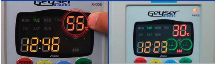
**2** Set the temperature per block to user requirements by using **▲** and **▼** arrow keys.
